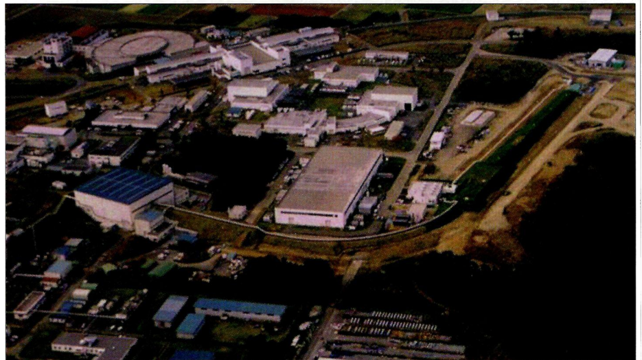
An aerial view of the K2K neutrino beamline at the Japanese KEK Laboratory. At the bottom left are the KEK 12 GeV Proton Synchrotron and its north counter hall. The extracted proton beam is bent around towards the near detector (small white building, top right) and exits towards Kamioka, 250 km away.
