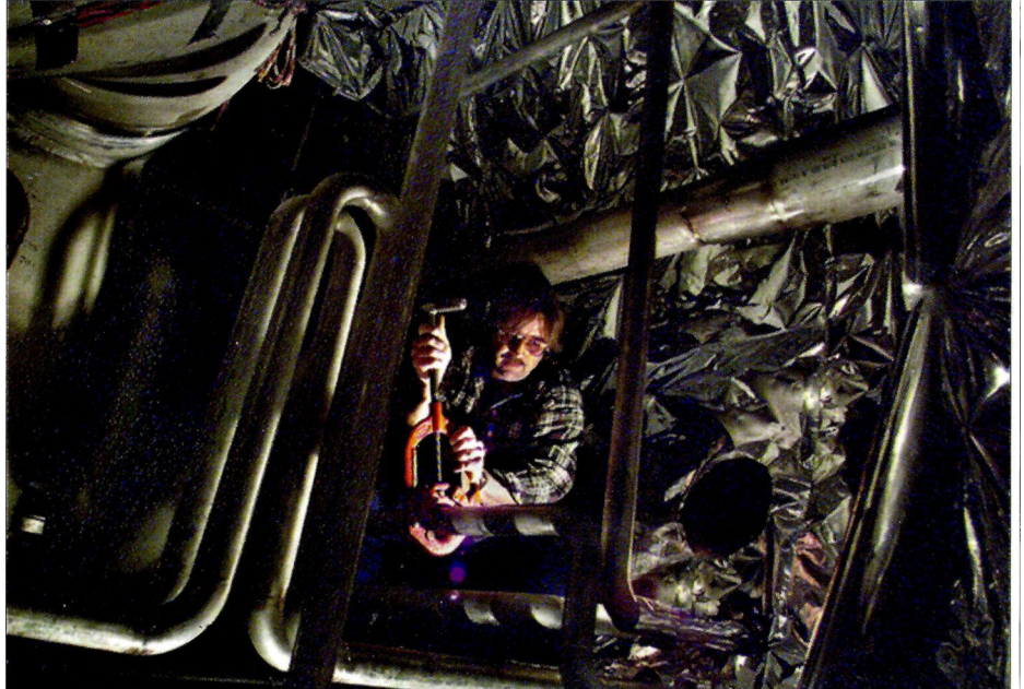
Work on the cryogenic system for Brookhaven's Relativistic Heavy Ion Collider. Equipped with superconducting magnets, the machine operates at 4.6 K. (R Stoutenburgh.)
